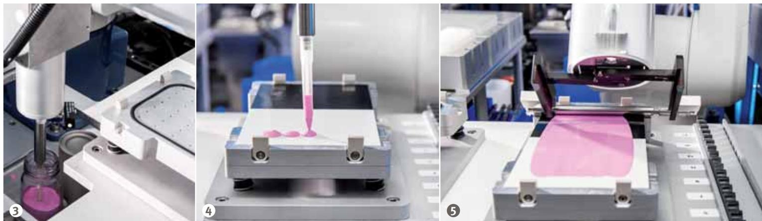
Figures 3, 4 and 5: Precise and cautious: A robot designed for this unique purpose draws the coating into a pipette, applies coating droplets onto a panel, and uses a doctor blade to produce a precisely defined coating thickness.
