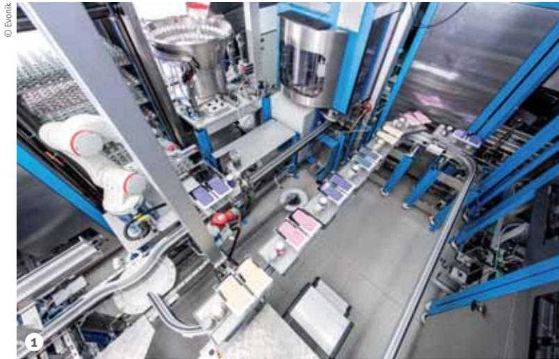
**Figure 1:** A track system for transporting panels and containers extends through the entire 120-square-meter HTE system.
