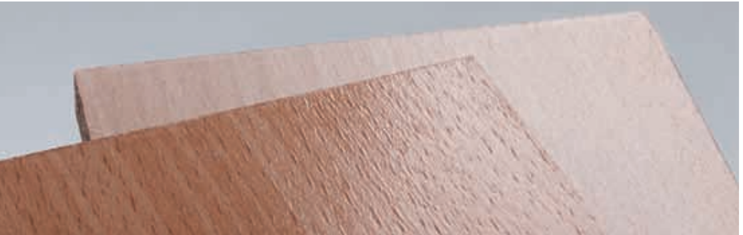
Figure 2: Waterborne wood coating, airless application
