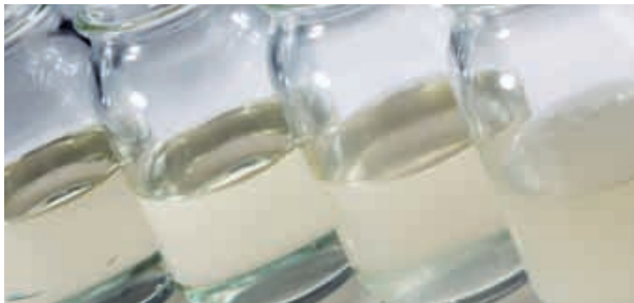
Figure 6: Solventborne clearcoat with different deaerators added: from left to right, completely soluble/insoluble/partially or targeted insoluble/incompatible
