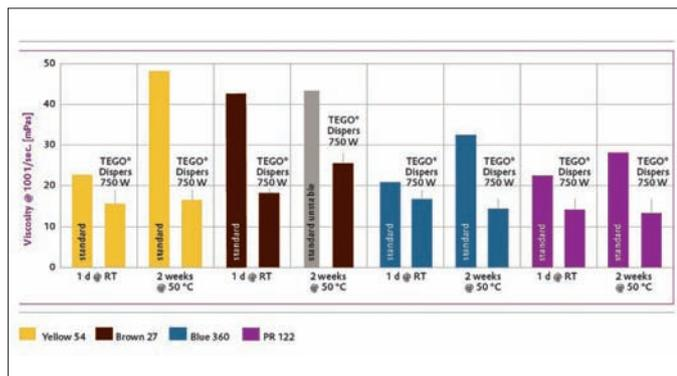
Fig.2: Viscosities determined according to DIN EN ISO 3219 using Anton Paar Model NCR 301, geometry CP50/2 at 23 °C and a shear ramp of 1 – 1000 1/sec.
