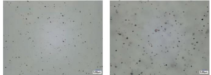
Fig. 3: KEYENCE VHX 5000 digital microscopic images of rub-outs with Brown 27 after one day storage at room temperature. Left: fine, homogeneous particles with high-performance wetting and dispersing agent (d50 = 294 nm). Right: coarse agglomerates with standard additive (d50 = 547 nm)
