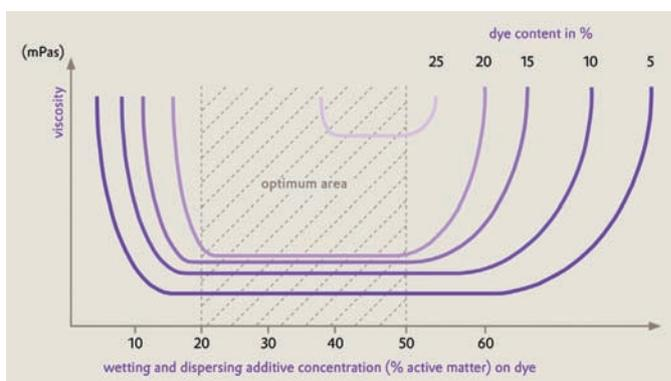
Fig 1: Influence of dye content and additive concentration on viscosity
