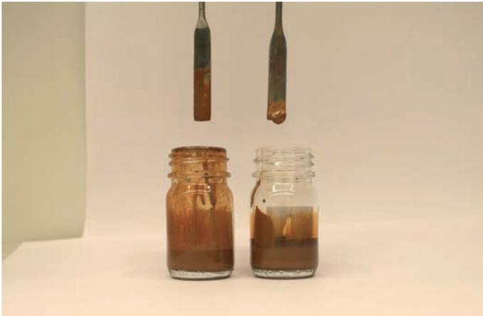
Fig. 5: Storage samples after 3 weeks at 50 °C of ceramic inks based on PB 28 with 45% solids content. Left: no settling with polymer wetting/dispersing additive ( $\eta = 21$  mPas at 1000 1 / sec.). Right: sediment with standard additive ( $\eta = 26$  mPas at 1000 1 / sec.)
