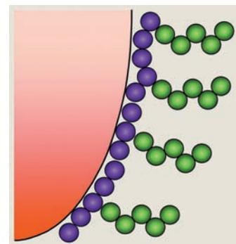
Fig. 4: Schematic representation of the anchoring of a graft copolymer on a colorant surface.
