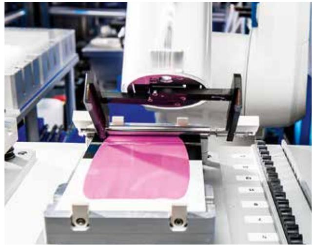
Precise and cautious: A robot designed for this unique purpose draws the coating into a pipette, applies coating droplets onto a panel, and uses a doctor blade to produce a precisely defined coating thickness.
