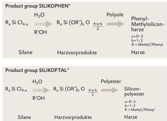
Figure 4: Resin manufacture at Evonik
