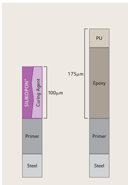
Figure 10: Coating structure
