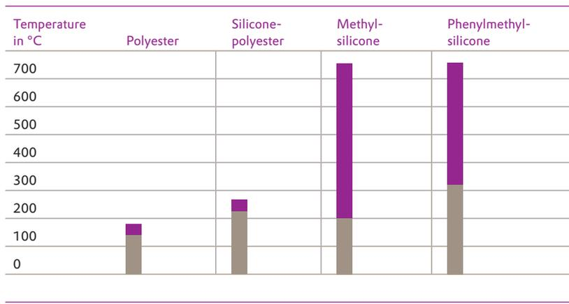
Illustration 1 ■ heat resistance as a function of pigmentation ■ continuous heat resistance
