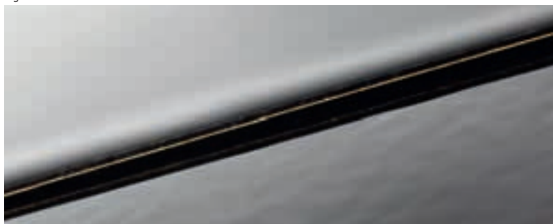
Figure 3: Surface texture with and without flow additive
