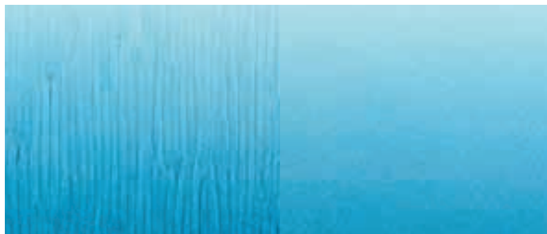
Figure 4: Matte clear-coat without additive (left) and with modified siloxane (right)
