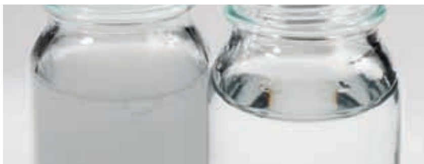
Figure 8: Clear coat with silicone oil (left) and with polyethersiloxane (right)
